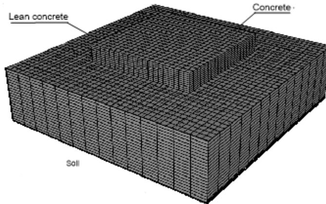
Figure 1. The calculation domain and finite volume mesh
