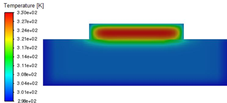
Figure 3. Distribution temperature in the foundation
