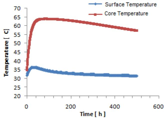
Figure 2. Minimum and maximum temperature inside the foundation
