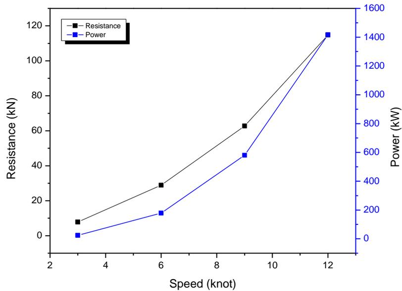
Figure 6. Ship Resistance – Ship Power Requirements
