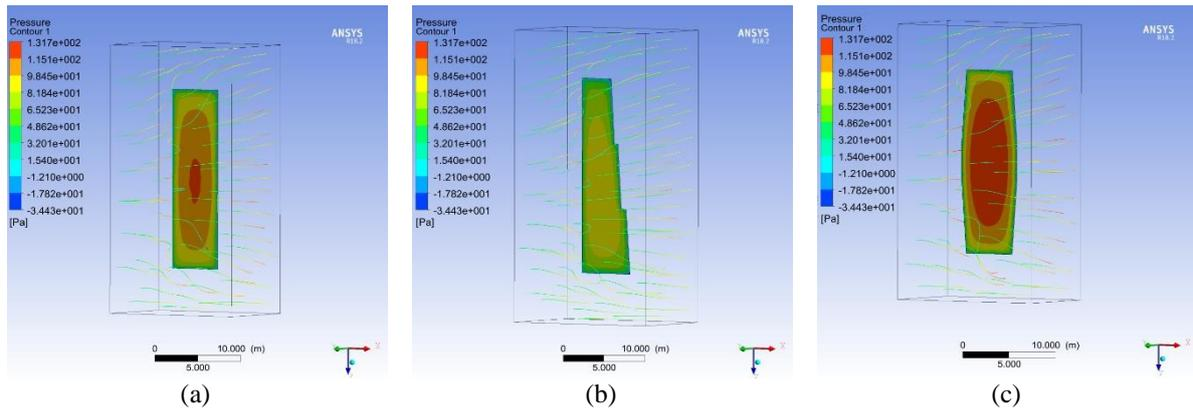
Figure 10. Simulation with Wind Direction Angle 0° (a) M<sub>1</sub>, (b) M<sub>2</sub>, (c) M<sub>3</sub>
