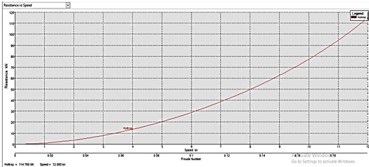
Figure 4. Graph of Resistance - Ship Speed
