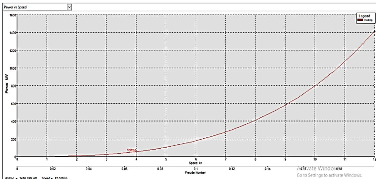
Figure 5. Graph of Ship Power - Ship Speed
