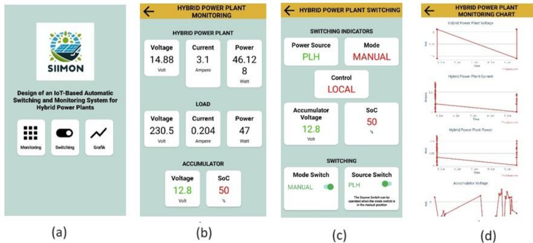
Figure 7. a. IoT Application Main Page, b. Hybrid Power Plant Monitoring Menu, c. Hybrid Power Plant Switching Menu, d. Hybrid Power Plant Monitoring Graph Menu
