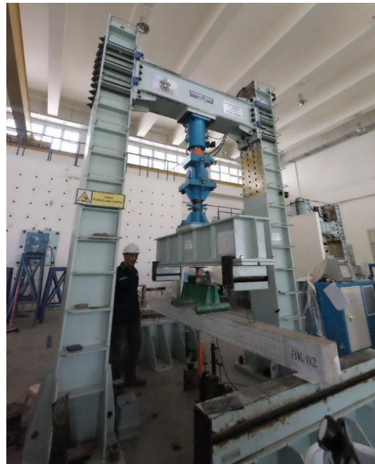
Figure 3. Example of Tests on Reinforced Concrete Beams
