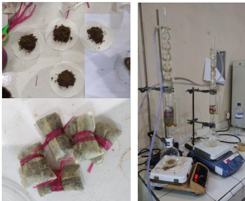
Figure 2. The Making of Sample Wraps and Soxhlet Extraction of BSF Larvae Oil
