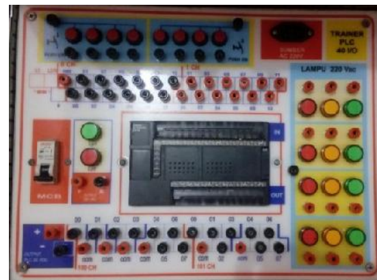
Gambar 8. Trainer PLC OMRON SYSMAC CP1E-E40DR-A
