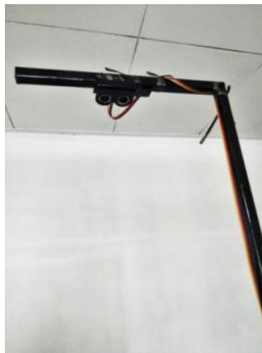
Figure 8. The position of ultrasonic sensor on the pole
