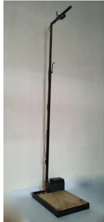
Figure 7. Instrument of body height and weight for a web-based anthropometry test
