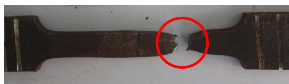
Figure 6. The Break Area in The Test Specimen
