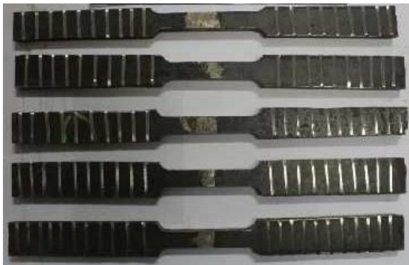
Figure 4. Low carbon steel test specimens according to ASTM E8-M standard
