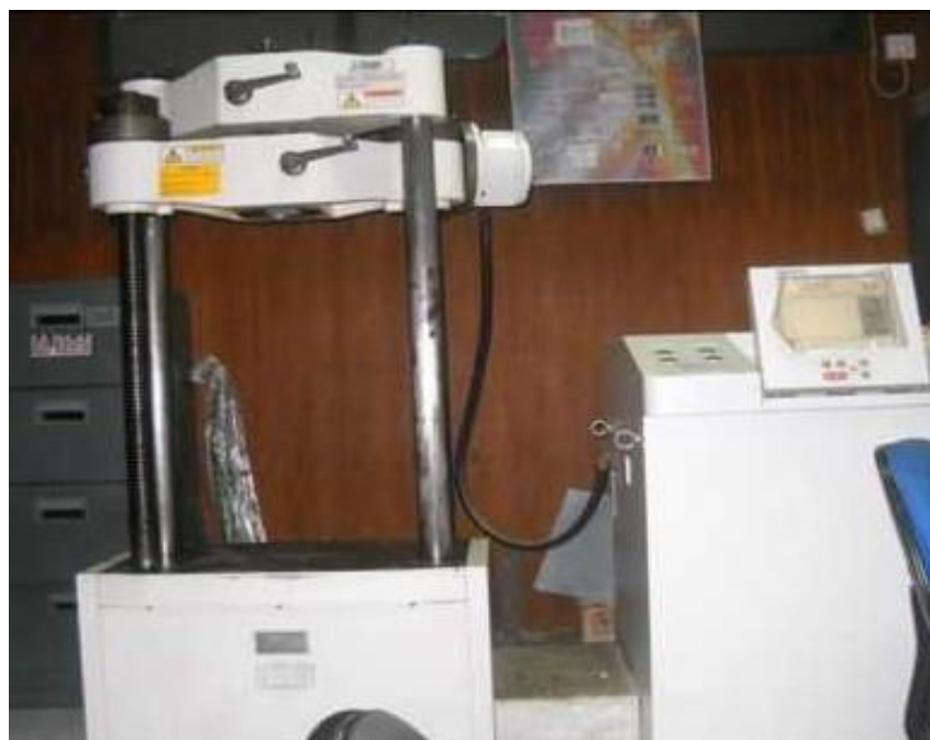
Figure 2. Shimadzu UH-300 kN type tensile testing machine
