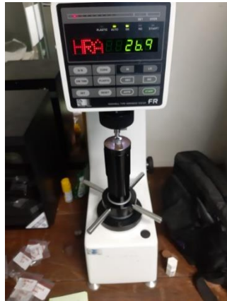
Figure 3: Rockwell hardness tester used
