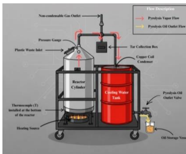
Figure 1. Experimental Setup of the Mixed Plastic Waste Pyrolysis System.
